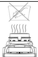
Make sure there are no heat sensitive or flammable material above the analyzer. The exhaust from the weighing chamber can be very hot.
