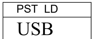
Press the **[Setup/Enter]** key to enter the test load function. The display will show the file name of the first test file found.
