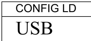
To recall any stored test procedure press the **[Dspl/ $\uparrow$ ]** key to show the configuration load screen.
