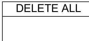
When the selection shows DELETE ALL, press **[Setup/Enter]** to delete all test results. The display will ask if you are sure you want to delete all results. Press **[Setup/Enter]** again. The display will count down from 99 to 0 during the time it takes to remove all the files.
