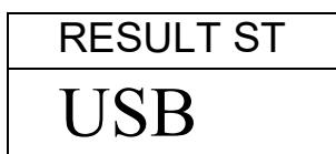
Press **[Setup/Enter]** to enter the test saving function. All of the test results stored in the analyzer memory will be copied to the USB memory. The file names will be the same as those used to store internally.
