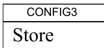
Press **[Setup/Enter]** to confirm the action. Or press **[→0/T← / Esc]** to escape back to the original USB display.
