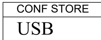
Press **[Setup/Enter]** to enter the configuration saving function. The display will show a suggested file name. The name will be the next logical name for the configuration file based on what data is already on the USB memory. For example if CONFIG1 and CONFIG2 are already stored, then it will display CONFIG3.
