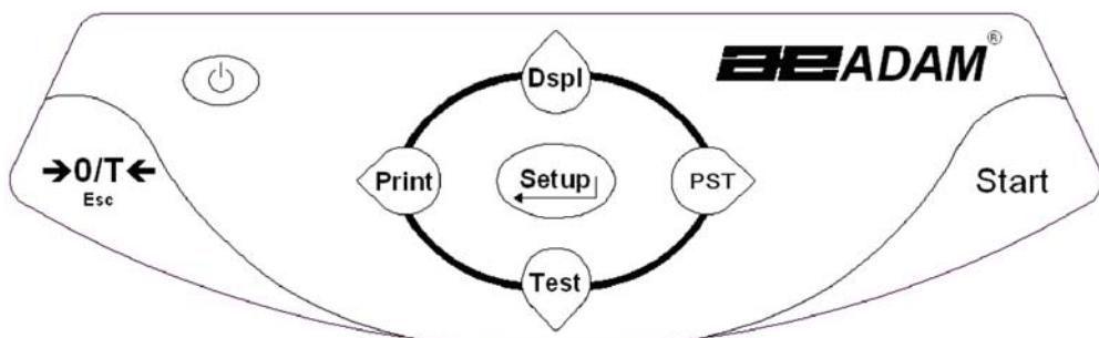
The keypad has second function keys to allow a selected menu item or value to be incremented or changed. Right/left shift to change the active digit and up/down to increment or decrement a value.
