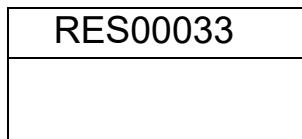
Press the **[Dspl/↑]** or **[Test/↓]** key to change the file name to the next available. When the desired test result is found press the **[Setup/Enter]** Key to delete just this file. The display will then show DELETED then the next available file. Press **[Setup/Enter]** to delete this file if desired.
